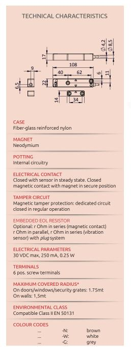
(\*) This is the maximum coverage when using VAS-series analysis boards. Coverage might decrease with other boards. Coverage might also be significantly affected by the door/window manterial, its type (fixed/openable), and the way it is fixed to walls. The same reasoning applies to the sensor's coverage area when mounted on walls.
