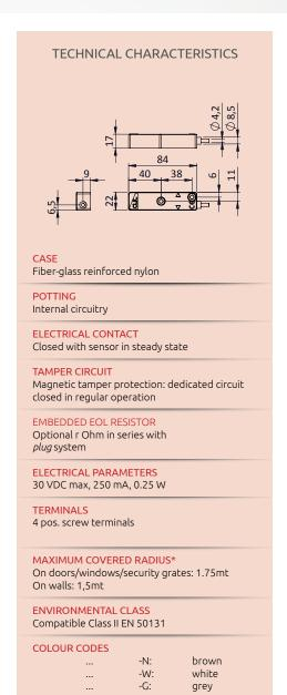
(\*) This is the maximum coverage when using VAS-series analysis boards. Coverage might decrease with other boards. Coverage might also be significantly affected by the door/window manterial, its type (fixed/openable), and the way it is fixed to walls. The same reasoning applies to the sensor's coverage area when mounted on walls.
