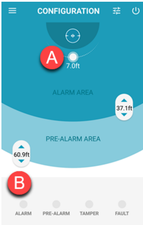
Wrong calibration. Calibration value too high.
